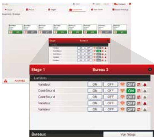
Lighting control and display: a global and detailed view of each zone
